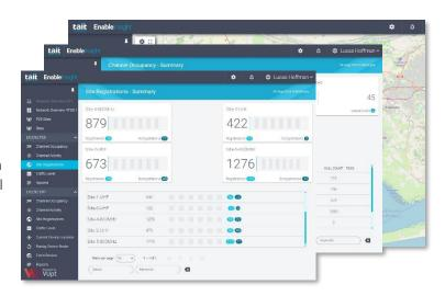
Tait EnableInsight analyses call activity on the customer network in near real-time and presents the users with information about current site loading, call queuing, and registration activity, as well as providing trend information over a range of timescales.
